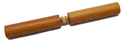
9. With the top part of the tool still on the pin of the bottom part of the tool, stand up the tool, holding it in one hand, pick up the hammer and pound on top of the top part of the tool to secure the eyelets in the center of the hole. Both should go in tightly at the same time!
